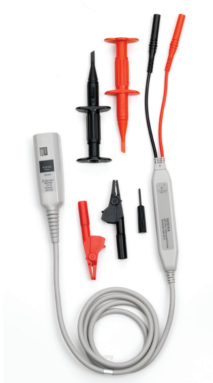
Figure 1: Keysight's N2818A 200-MHz differential active probe.
